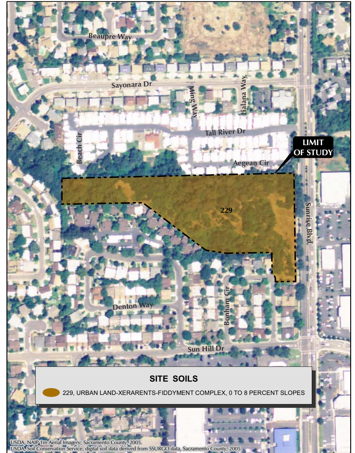
SOILS 229, URBAN LAND-XERARENTS-FIDDYMENT COMPLEX, 0 TO 8 PERCENT SLOPES FOOTHILL ASSOCIATES ENVIRONMENTAL CONSULTING • PLANNING • LANDSCAPE ARCHITECTURE Scale: 0 150 300 SCALE IN FEET Drawn By: MJ Date: 03/26/08 FIGURE 2
