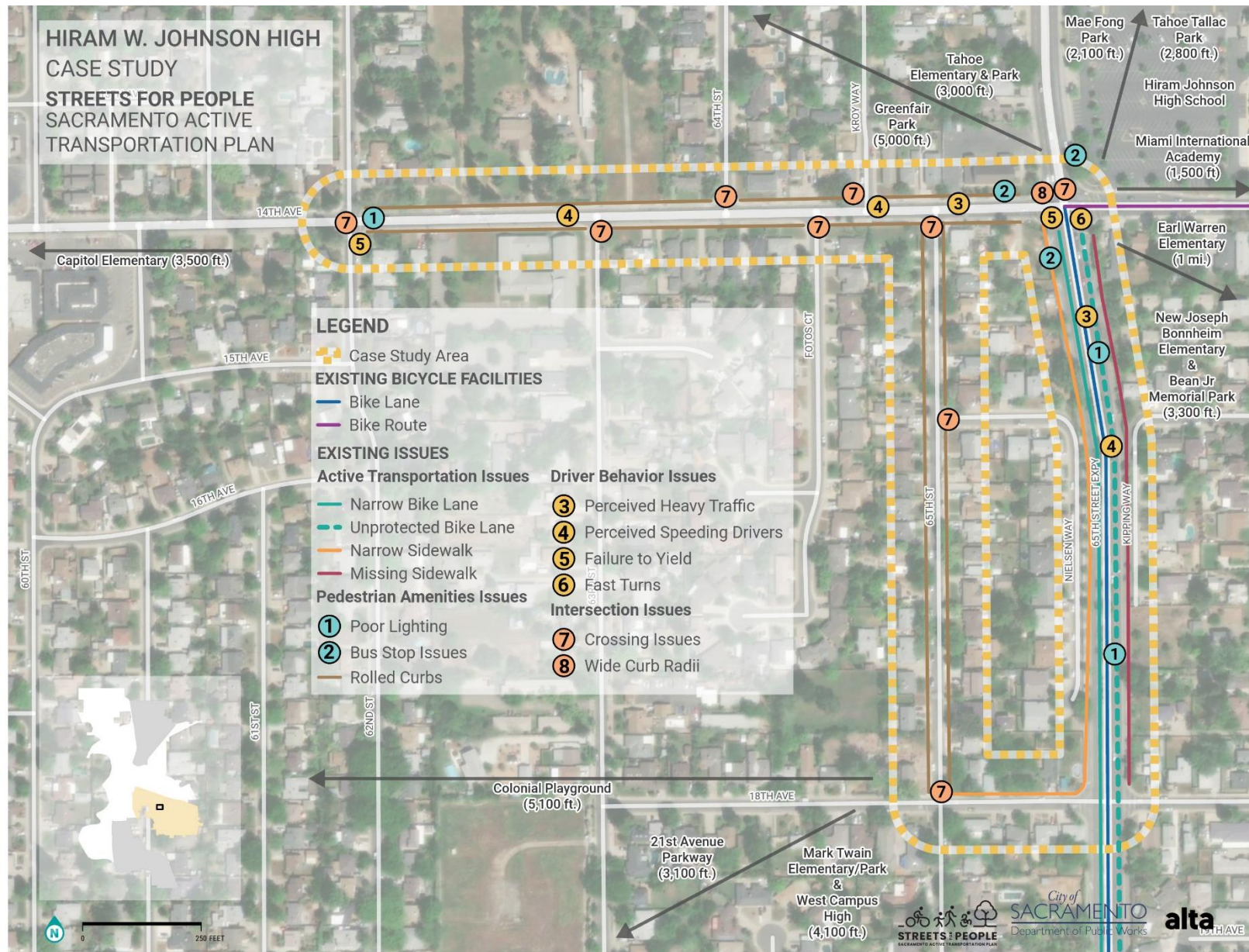
Figure 25. Hiram W. Johnson High School Case Study Area – Documented Issues
