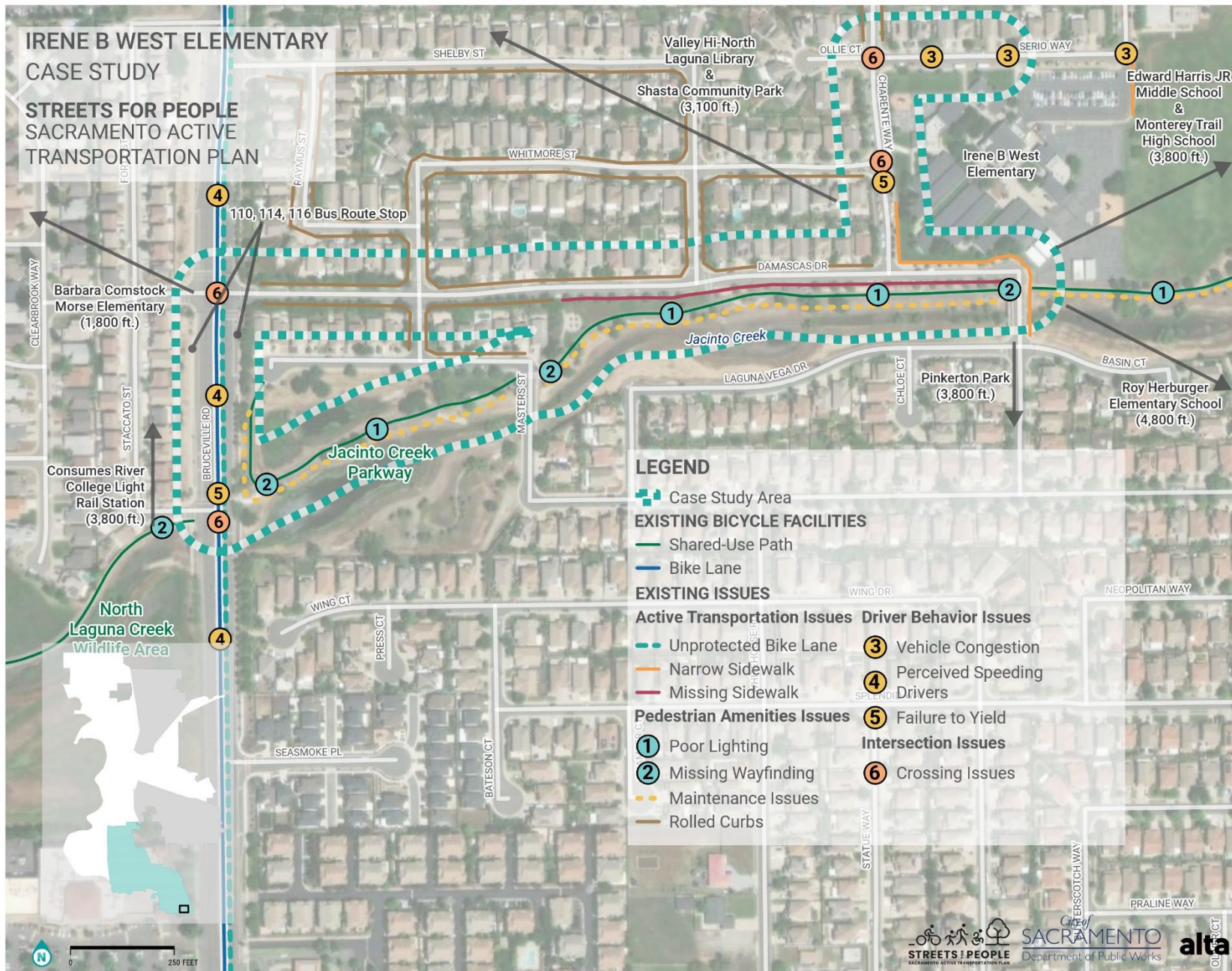
Figure 49. Irene B. West Elementary School Case Study Area – Documented Issues
