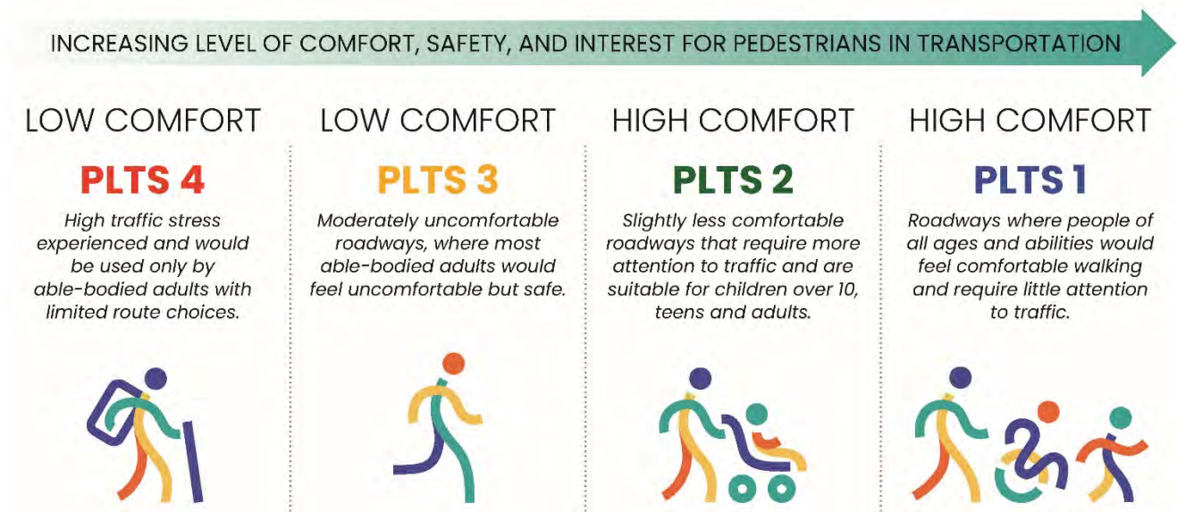
Figure 15. Pedestrian Level of Traffic Stress Illustrated
