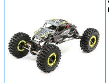
A remote-controlled, uncrewed vehicle that operates on the ground. Modified and equipped by the department with a camera.
