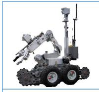
A remote-controlled, uncrewed machine that operates on the ground. A heavy-duty robot, with stair climbing ability and an arm capable of lifting 65 pounds.
