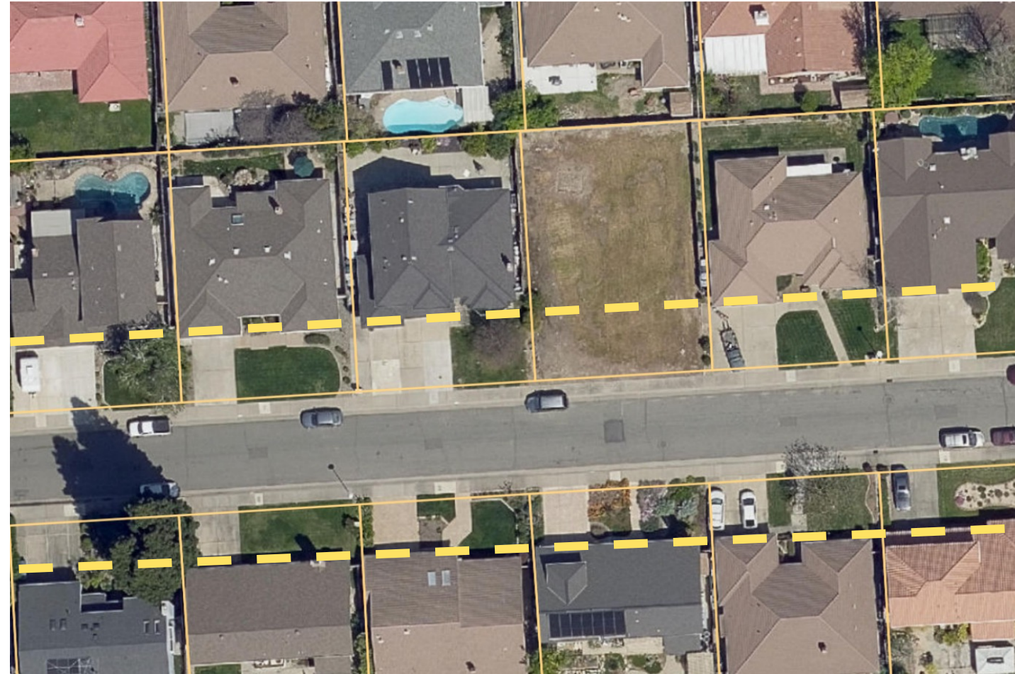
Typical condition with 20 ft setback. Not all front setbacks have active frontages.
